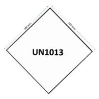
The "UN 1013" marking must be displayed within a square-on-points shaped area surrounded by a line that measures at least 100mm by 100mm on each side. When the
