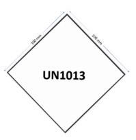
The "UN 1013" marking must be displayed within a square-on-points shaped area surrounded by a line that measures at least 100 mm by 100 mm on each side. When the package dimensions are such that the 100 mm mark cannot be accommodated, the mark may be proportionately reduced to the largest possible dimensions that can be accommodated. The minimum measurement allowed is 30 mm on each side.
