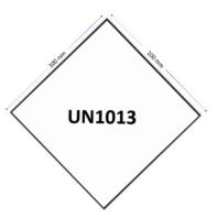
The "UN 1013" marking must be displayed within a square-on-points shaped area surrounded by a line that measures at least 100 mm by 100 mm on each side. When the package dimensions are such that the 100 mm marking cannot be accommodated, the marking may be proportionately reduced to the largest possible dimensions that can be accommodated. The minimum measurement allowed is 30 mm on each side.
