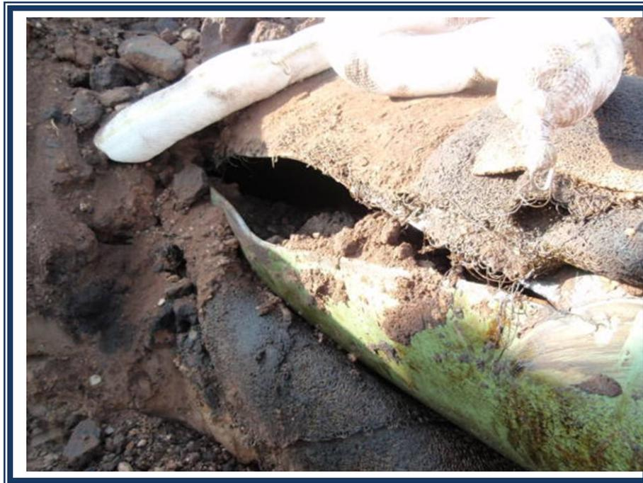
Figure 1 – Failed Pipe Joint
